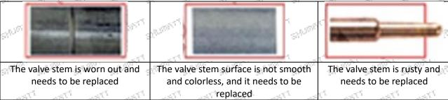
▲ The excessive clearance between the stem wear and the housing and between the cap causes an injector
